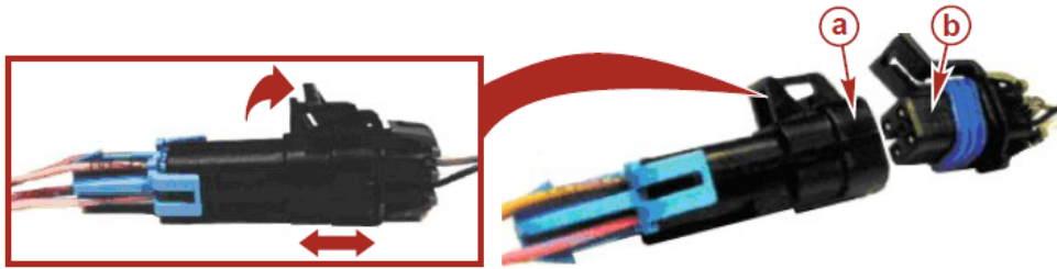
Figure 7 - Four wire oxygen sensor connector, "a" is the engine harness connector and "b" is the sensor connector
