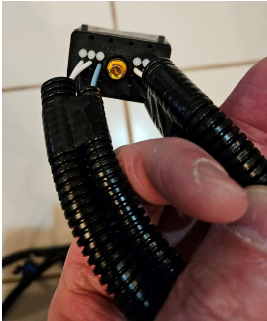
Figure 3- The connector that attaches to the computer has an attaching screw with a \frac{1}{4} " head.
